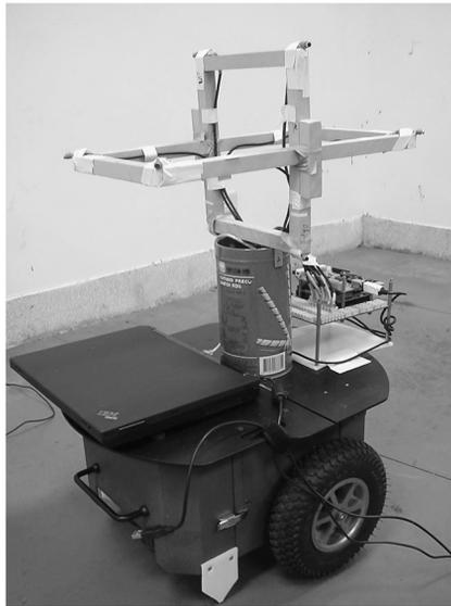
**Figure 2.** Digital microphone array mounted on the robot.
