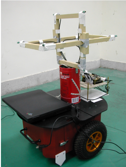
Fig. 2. Digital microphone array mounted on the robot
