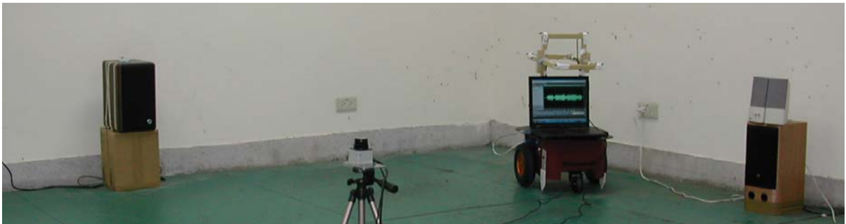
Figure 12. The Spatial Relation of the Speaker, the Robot, and the Laser Range Finder
